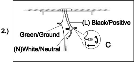
Step 2:Adjust wires to desired mounting height. Wire fixtures to wire in outlet box. Refer to dual plastic wire instructions to connect low voltage wire to driver.
