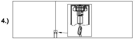
Tighten the top lid on the tube using the fork tool provided until flush.
