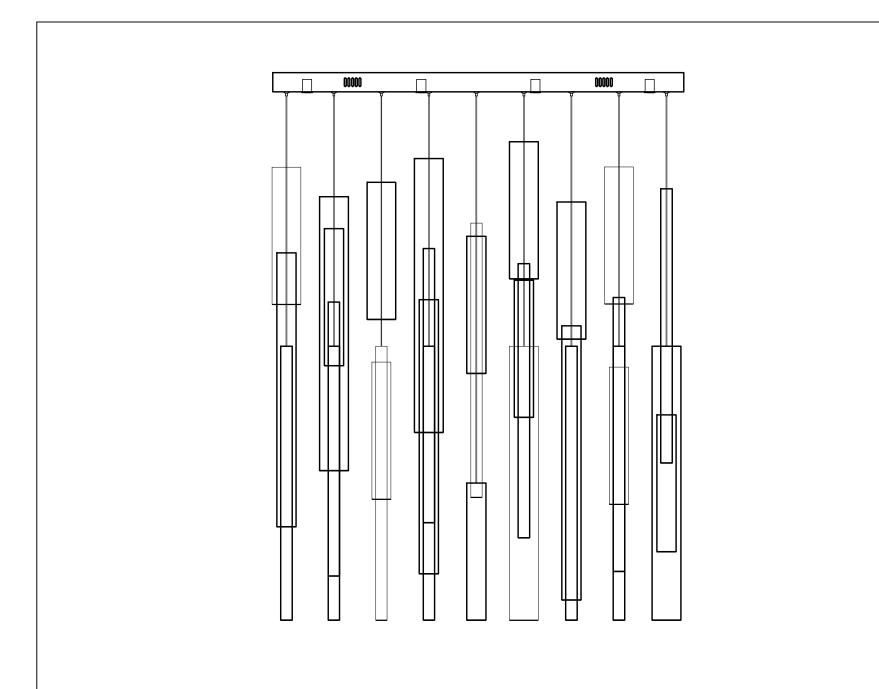
WARNING: Wires need to be connected to driver found in canopy and should not be connected directly to power source or a short may occur.
