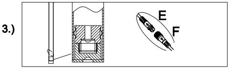
Run the wire through the tube and plug in (E) and (F) following the direction of written on the plug.
