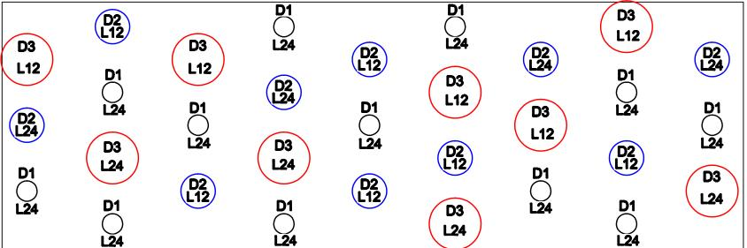
Please check the label on wire and label on pipe to find correct pipe for install, eg. A wire with D3, L12 label should connect to a pipe that with D3 L12 label on it.
