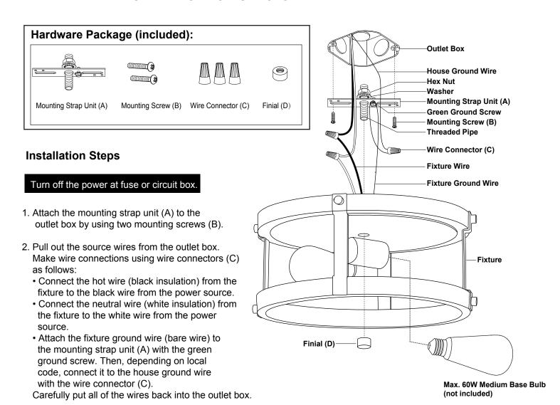
3. Attach the ceiling pan to the mounting strap unit (A) by inserting threaded pipe into the center hole the ceiling pan and secure it with the finial (D).
