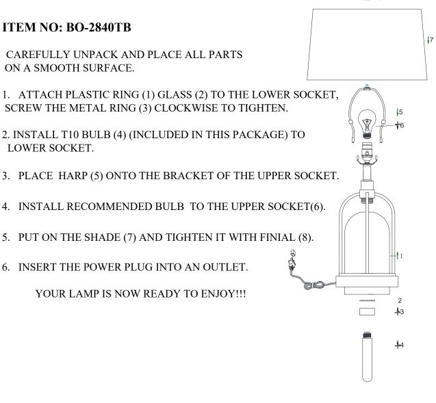
Use 100W Max type A bulb (bulb not included) and 25W Max T10 bulb (bulb included)
