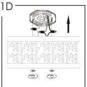
Lining up threads on mounting plate with holes in fixture pan, attach fixture to junction box using cap nuts. Be sure to carefully tuck wires into pan while attaching.
