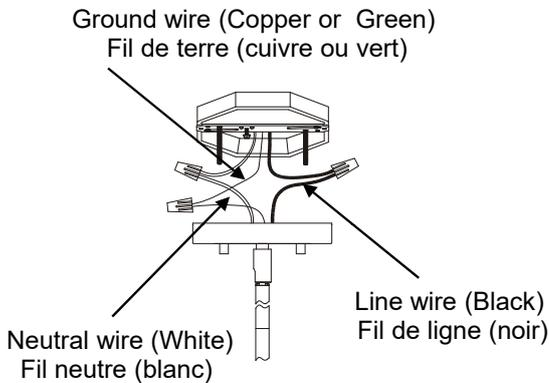
Connect the **GROUND WIRE** from junction box to **GROUND** (or **GREEN**) wire from fixture with a wire nut. Connect the **NEUTRAL WIRE** from junction box to **NEUTRAL** (**WHITE**) wire from fixture with a wire nut. Connect the **LINE WIRE** from junction box to **LINE** (**BLACK**) wire from fixture with a wire nut.
