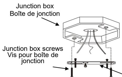
Attach the mounting bracket to junction box with screws provided.
