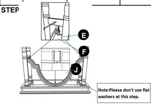
Attach wooden supporter to the unit with bolts "F" "J", flat washers and Allen wrench "H".Please don't fully tighten bolts.
