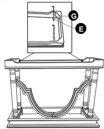
Attach wooden base to the end of leg with bolts "G" , flat washers and Allen wrench "I".
