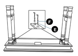
Put the table top upside down on soft & clean surface. Attach metal leg to the bottom of the table top with bolts" F ", flat washers and Allen wrench "H" as shown above. Please don't fully tighten bolts.
