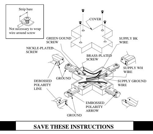
NOTE : Put BK and WH jumper wire as the picture shows to complete the circuit in this X connector.
