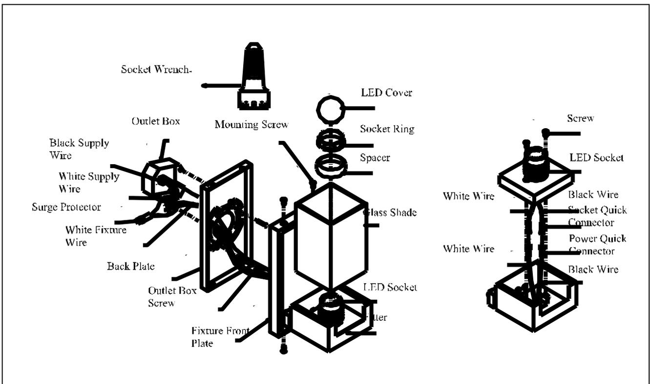
Line art shown may not exactly match the fixture enclosed. However, the installations do apply to this fixture. ITEM NO:1920-1S
