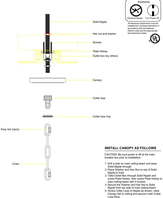
6. Hang Chain to Collar Loop with the Easy Link, Proceed to fixture frame assembly Step 1.
