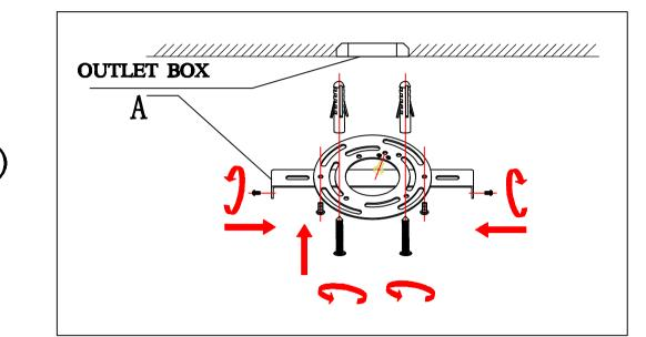
Step.1: Remove Mounting Bracket (A) from Canopy to install to electrical box.
