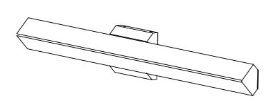
LA-8605-S: 13W Max LED LA-8605-M: 26W Max LED LA-8605-L: 39W Max LED
