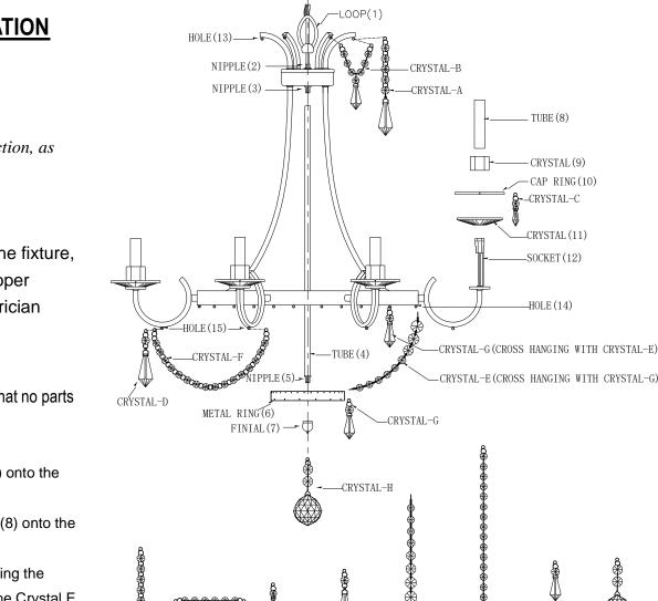
CRYSTAL-C CRYSTAL-E CRYSTAL-G CRYSTAL-H CRYSTAL-D CRYSTAL-F CRYSTAL-B CRYSTAL-A 26PCS 7PCS 7PCS 37PCS 51PCS 1PCS 6PCS 6PCS (INCLUDING (INCLUDING (INCLUDING (INCLUDING (INCLUDING SPARE PARTS SPARE PARTS SPARE PARTS SPARE PARTS SPARE PARTS 2PCS) 1PCS) 3PCS) 1PCS) 3PCS)
