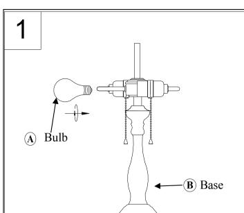
Screw on the bulb (A) make sure this is done with the power off.
