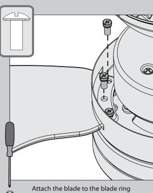
Attach the blade to the blade ring using the blade assembly screws, found in the **A** hardware bag.
