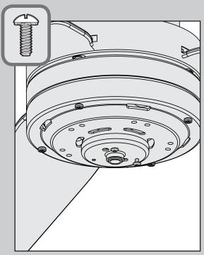
Partially install two machine screws, found in the ≡ hardware bag, halfway into the motor housing. It does not matter which two screw holes you choose.
