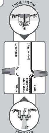
Using the orange wire connectors from the \*\frac{\stack}{} hardware bag, connect the black wire (ungrounded) from the ceiling to the black and the black with white stripe wires from the fan. Connect the white wire (grounded) from the ceiling to the white wire from the fan.
