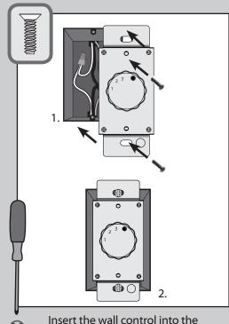
outlet box and secure the two metal tabs to the tabs on the switch box using the two flat head screws that came with the switch box.
