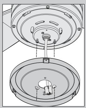
Feed the wires through the center hole of the upper switch housing, then wrap the keyhole slots around the screws and twist counterclockwise.
