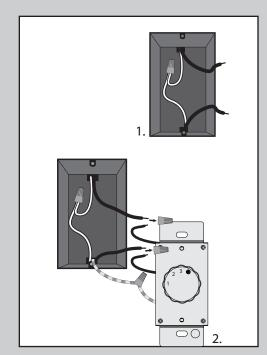
Using the wire connectors, connect each black wire from the wall control to a black wire from the switch box. Connect ground wire from the switch box to the green/yellow wire from the wall control.
