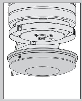
Raise the bottom cap to the switch housing. Align the screw holes in the switch housing and the screw holes in the bottom cap.
