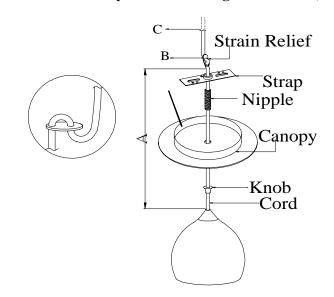
**2**. Within the length of 1-1/2" D on the cord from the top, make a mark E, use knife to slightly cut the cord and then peel off the length of cord outside D and leave 3 wires inside.
