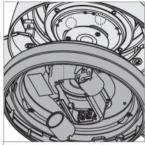
Align the keyhole slots in the top of the upper switch housing with the partially installed light kit screws. Wrap the keyhole slots around the screws and twist counterclockwise
