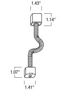
NT-330B: Black 18" Flexible Extension Rod NT-330W: White 18" Flexible Extension Rod
