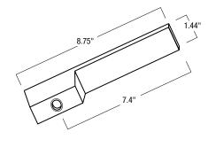
NT-326B: Black Wire Way Cover NT-326S: Silver Wire Way Cover NT-326W: White Wire Way Cover
