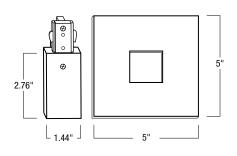
NT-2311B: Black Live End Feed with Canopy NT-2311S: Silver Live End Feed with Canopy NT-2311W: White Live End Feed with Canopy
