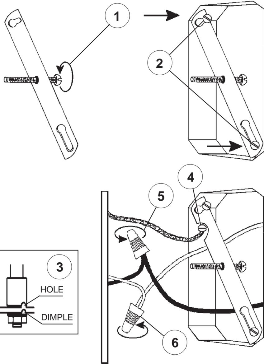
Turn arms to line up holes in arms with dimple in plate. Tighten lock washer and nut to secure arms in place.
