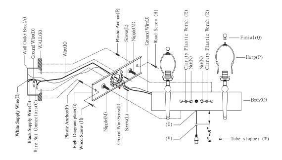
tube stopper (W) to replace wire clap at point (U).
