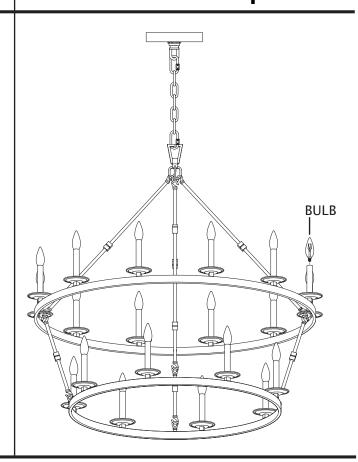
28. Screw recommended bulbs (E12 Candelabra bulb type, not included) into sockets. Verify correct bulb wattage marked on socket of fixture. **WARNING:** DO NOT exceed maximum bulb wattage
