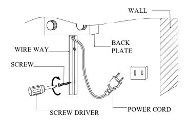
4. Attach wire way or more wire ways to be connected on the wall by screws provided.
