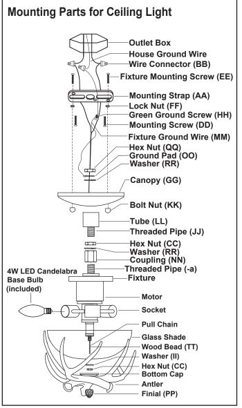
The following parts are available for reorder if damaged or missing.
