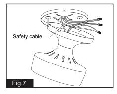
Hang the safety cable into the safety cable hook.
