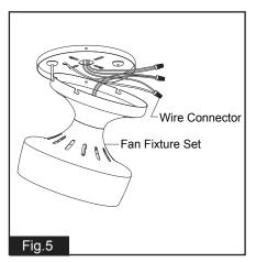
Make wire connections: 1).The white motor wire to the white wire from the outlet box with a wire connector.
