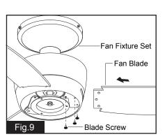
Insert the fan blade through the slot on the fan fixture set. and fasten fan blade to the fan fixture set with screws. Repeat for remaining fan blades.
