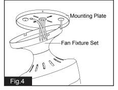
Left fan fixture set and hang on mounting plate with hook provided, through one of the two holes in canopy. This will allow for hands-free wiring. CAUTION: Use only a side with hole in canopy, not hook slot.
