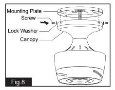
Position both slots on the canopy directly under and in line with two screws and lock washers in the mounting plate. Lift the canopy, allowing the two screws and lock washers to slide into the mating slots. Rotate the canopy counterclockwise until both screws from the mounting plate drop into the slot recesses. Tighten screws securely. Install the other two screws and lock washers into the mating holes of the mounting plate and tighten to secure the canopy to the mounting plate.
