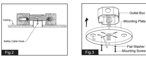
Screw the safety cable hook to the ceiling outlet box. Insert wires from the outlet box through the hole in center of mounting plate. Attach the mounting plate to the outlet box by using two flat washers and mounting screws. WARNING: MOUNT ONLY TO AN OUTLET BOX MARKED " ACCEPTABLE FOR FAN SUPPORT OF 15.9KG(35LBS) OR LESS"!
