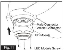
Make wire connection. Plug the male connector from the motor into the female connector from the LED Module . Carefully put the wires into the switch box. Secure the LED Module up to the bottom of the motor with LED Module screws.
