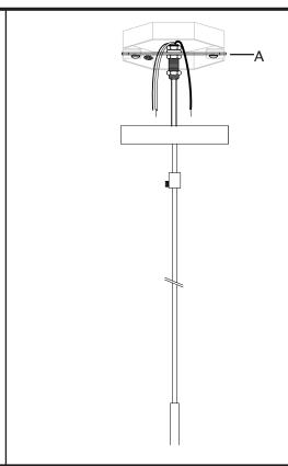
10. Slightly loosen ground screw on mounting bracket (A). Do not completely remove ground screw. Wrap ground wire from junction box around ground screw, leaving enough ground wire to attach to fixture ground wire. Twist end of fixture ground wire and end of house ground wire together. Twist wire nut (C) onto ends of wires. Completely tighten wire nut (C). Reference chart below for correct wire connections.
