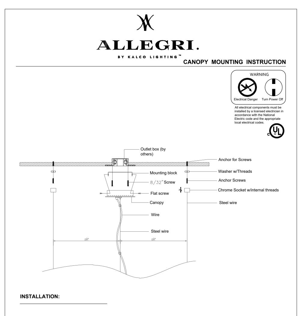
1. Install anchor screws as shown in diagram at 15 3/4" from center of
