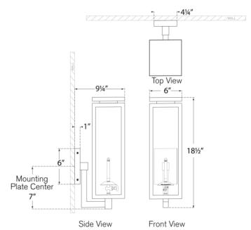
Gas light fixture supplied with 3/16"copper gas line and 3/16" x 1/4" gas line adaptor
