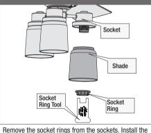
shades onto the sockets. Install the socket rings onto the sockets. Tighten them by turning clockwise with the socket ring glass tool.
