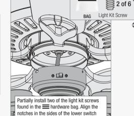
housing with the screws on the upper switch housing. Twist the lower switch
