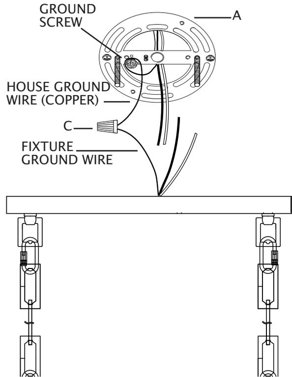
17. Twist end of house lead wire (black) and end of fixture lead wire together. Twist wire nut (C) onto ends of wires. Completely tighten wire nut (C). Twist end of house neutral wire (white) and end of fixture neutral wire together. Twist wire nut (C) onto ends of wires. Completely tighten wire nut (C). Reference chart to the right for correct wire connections.
