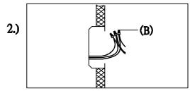
Step.2: Wire fixture to wires (B) in outlet box. Copper wire is for Ground.
