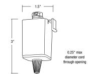
NT-368B: Black Pendant Track Adapter NT-368S: Silver Pendant Track Adapter NT-368W: White Pendant Track Adapter NT-368B/J: Black Pendant Track Adapter (Juno Compatible) NT-368S/J: Silver Pendant Track Adapter (Juno Compatible) NT-368W/J: White Pendant Track Adapter (Juno Compatible)
