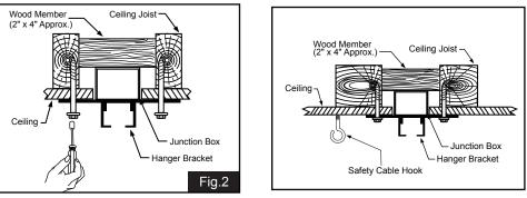
Tighten the hanger bracket to the outlet box with two mounting screws.(**Make sure the outlet box is securely installed so that it will be able to support at least the fan weight.**) Attach the safety cable hook to the ceiling, and make sure the safety cable hook is covered by the fan canopy. **WARNING: MOUNT ONLY TO AN OUTLET BOX MARKED "ACCEPTABLE FOR**
