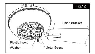
Remove the motor screws, plastic inserts and washers from the fan motor assembly. Secure blade brackets to the motor with washers and motor screws.
