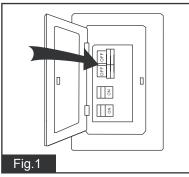
Turn OFF the electric circuit at the main fuse or circuit breaker box.
