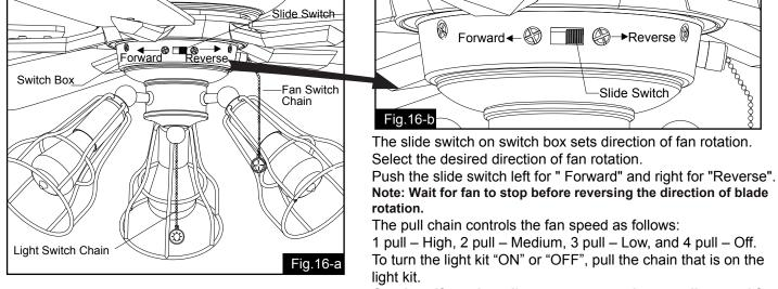
Caution: If you install a remote control or a wall control for this fan, pull the pull chains to "high speed" of the fan motor and "on" of the fan light.
