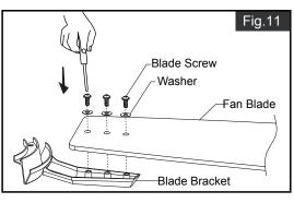
Tighten fan blades to blade brackets by using washers and blade screws.
