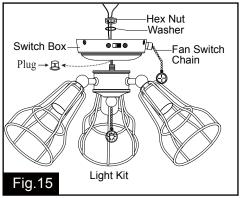
Remove the plug from the switch box. Remove the nut and lock washer from light kit. Attach the light kit to the switch box by threading the light kit wires (black and white) and the
