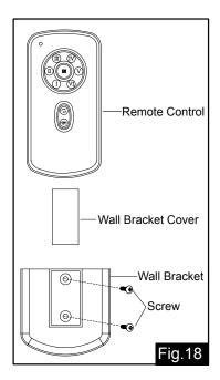
Slide off the wall bracket cover from the wall bracket. Install the wall bracket on a wall with the two screws included. Place the wall bracket cover back on the wall bracket to cover the screws. Slide the remote control into the wall bracket.
