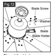
Thread the blade screws through the washer, blade into blade holder. Tighten all blade screws securely. Repeat to other blades.
