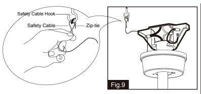
Hang the safety cable into the safety cable hook, tighten the safety cable to the safety cable hook by using the zip-tie.
