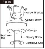
Remove one canopy screw (for later use), then push the canopy upwards by inserting canopy screw head left in hanger bracket into key hole slot, rotate the canopy till the hole in canopy aligns the hole in hanger bracket, finally, secure the canopy to hanger bracket with
