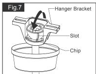
Hang the fan on hanger bracket, and make sure the slot of hanger ball is snapped into the chip of hanger bracket exactly.
