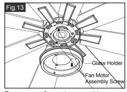
Remove one fan motor assembly screw (for later use), push the glass holder upwards until the fan motor assembly screws insert into the key hole slot of glass holder then rotate the glass holder till it is fixed on the motor bottom. Finally, secure the glass holder to motor bottom with previous screw which we removed and tighten the other two fan motor assembly screws.
