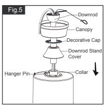
Loosen the collar screws out part way. Insert the downrod into the collar. Slide hanger pin through holes of collar and downrod.
