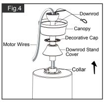
Thread the motor wires through the downrod stand cover, decorative cap (Making sure the smooth side of decorative cap is facing downward.), canopy and downrod.
