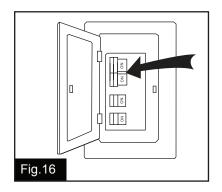
Turn ON the electric circuit at the main fuse or circuit breaker box.
