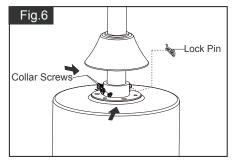
Tighten the two collar screws. Slide lock pin into hanger pin until it is locked into position.
