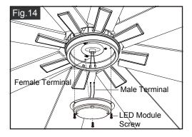
Connect the female terminals from motor to male terminals from LED module.
