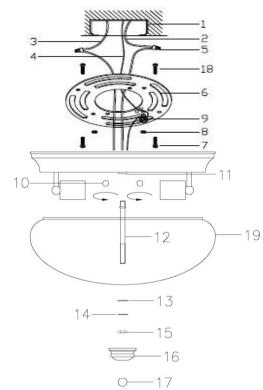
1. OUTLET BOX 2. WHITE WIRE 3. BLACK WIRE GROUND WIRE 5. WIRE CONNECTOR MOUNTING BAR 7. MOUNTING SCREW 8. HEX NUT 9. GROUND WIRE SCREW 10. BALL NUT **11. CONNECTOR** 12. NIPPLE **13. RUBBER WASHER 14. FLAT WASHER** 15. HEX NUT 16. CAP **17. FINIAL 18. MOUNTING SCREW** 19. GLASS
