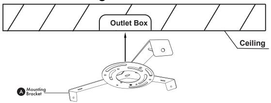
Align mounting bracket (A) with outlet box.
