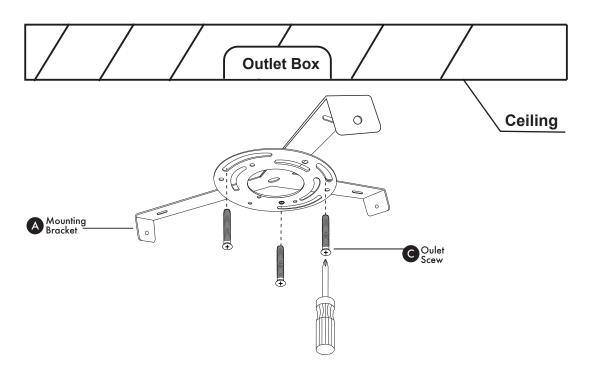
Attach mounting bracket (A) to outlet box. Secure with outlet screws (C).
