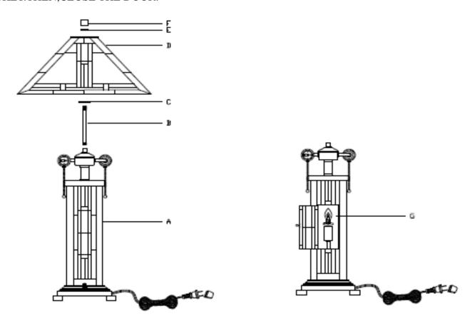
Recommended (2) maximum 60 WATT Type "A" Bulbs Or (2) maximum 13WATT CFL Bulbs (Bulbs not included) for Top light.
