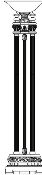
1. Carefully pull cord outward from base (D). Pull cord taut. Screw center tube (E) onto top of base (D).
